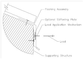
Figure 1 – Single Load Test Apparatus
