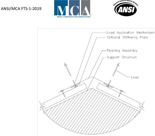
Figure 3 – Two Load Test Apparatus
