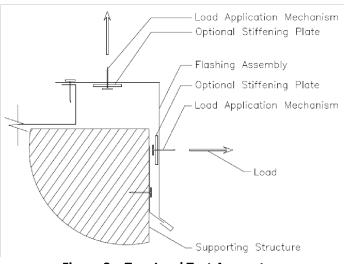
Figure 2 – Two Load Test Apparatus
